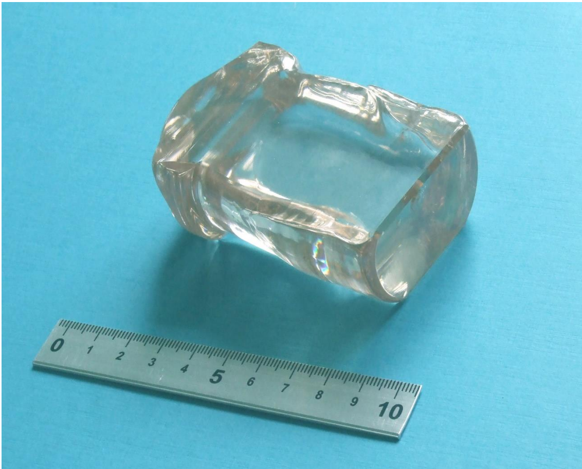
Fig. 1 The crystalline boule mixed (\text{Zn}_{0.9}\text{Cd}_{0.1})(\text{W}_{0.9}\text{Mo}_{0.1})\text{O}_4 crystal
